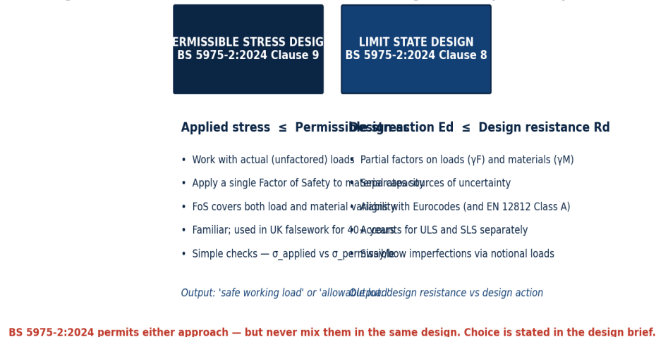
Figure 6.1 — Permissible Stress and Limit State Design — Conceptual Comparison
